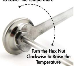
NOTE: This image has the thermometer upside-down just to demonstrate where the hex nut is actually located - you will want to be looking at the dial face to determine whether you are spinning the nut clockwise or counter-clockwise.
