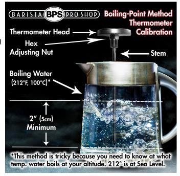
Compare the temperature reading to the temperature at which water boils for your eleveation and adjust your thermometer as needed.
