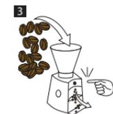
Flush out remaining tablet dust by grinding a handful of coffee beans
